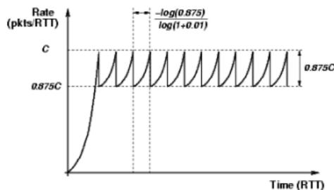
Figure: Packet loss recovery times for the traditional TCP (left) are proportional to  $cwnd$  and RTT. A Scalable TCP connection (right) has packet loss recovery times that are proportional to connection's RTT only. (**Note:** link capacity  $c < C$ )
