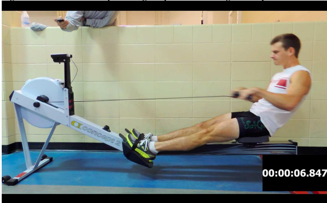
Figure 8: When the seat stops moving. Stop time for average velocity of the seat.
