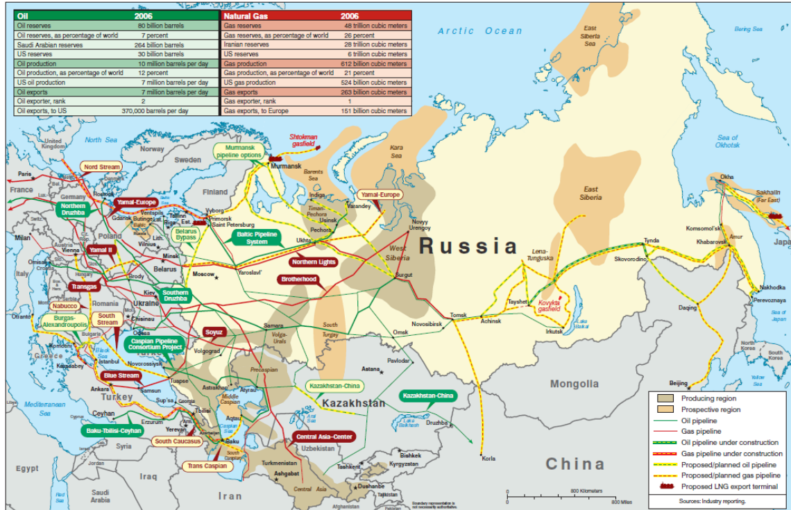
Figure 1: The logistics infrastructure of oil and the natural gas from Russia
