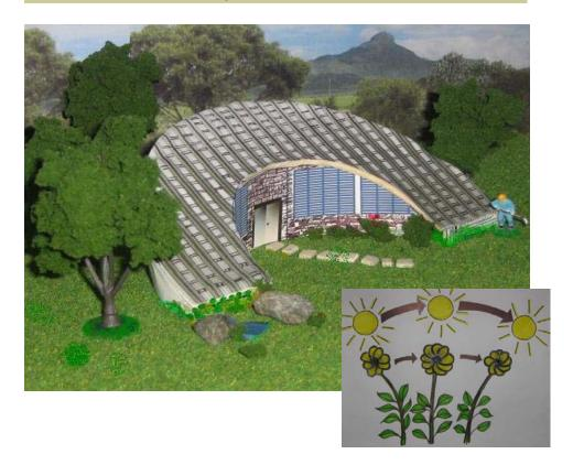
The Heliotropic House mimics sun-tracking plants in order to maximize collection of solar rays. It's slightly concave, semi-circular roof is paneled with solar cells and also channeled with grooves to collect water. The collected solar energy can be used to power the home and the collected water is stored in tanks for later use.
