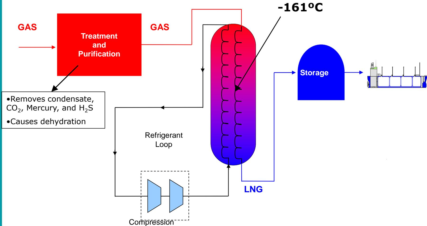
Purified gas is cooled to minus 161 C at which temperature it becomes a liquid at atmospheric pressure. Volume reduced by a factor of 600 compared to gas at atmospheric pressure.
