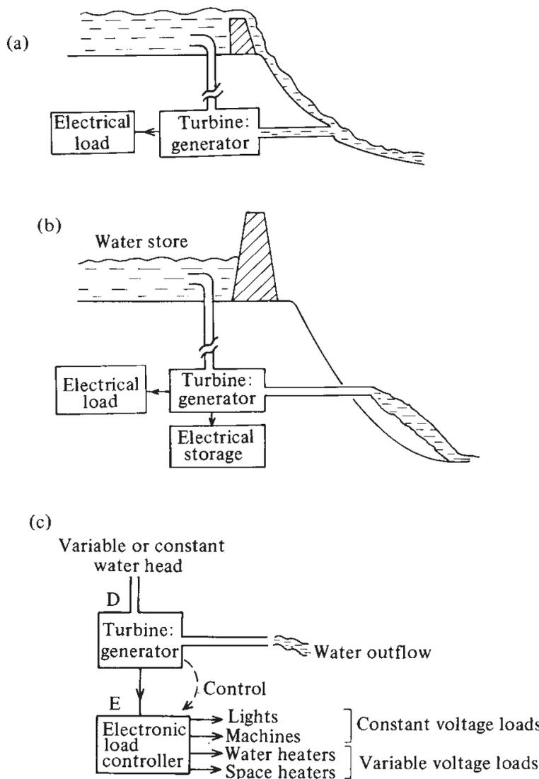
Figure 1.5 Examples of control. (a) Control by spilling excess energy: constant pressure maintained for the turbine. (b) Control incorporating storage in hydroelectric catchment dam. (c) Control by load variation: feedforward control. Load controller automatically shunts power between end-uses, maintaining constant generator load at E. Turbine also has constant load and hence constant frequency: only rudimentary mechanical control of turbine is needed.
