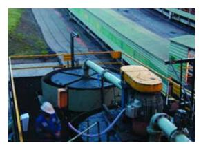
Froth flotation cells at Goedehoop Colliery are used for fine coal beneficiation. Photograph courtesy of Anglo Coal. Measures are taken at every stage of coal transportation and storage to minimise environmental impacts (see Section 5 for more information on coal and the environment).
