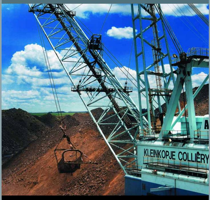
Large opencast mines can cover an area of many square kilometres and use very large pieces of equipment, such as draglines (pictured here). Photograph courtesy of Anglo Coal. SECTION TWO
