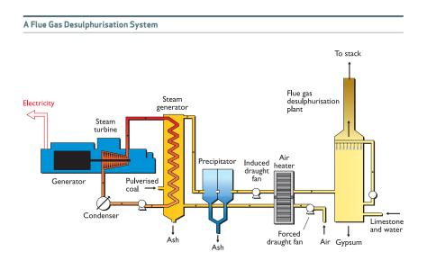
electrostatic precipitators remove 99.8% of fly ash, some of which is sold to the cement industry. For Eskom, the plant operator, the use of ESPs has had a major impact on the environmental performance of its power stations. Between 1988 and 2003, it reduced particulate emissions by almost 85% while power generated increased by over 56%.
