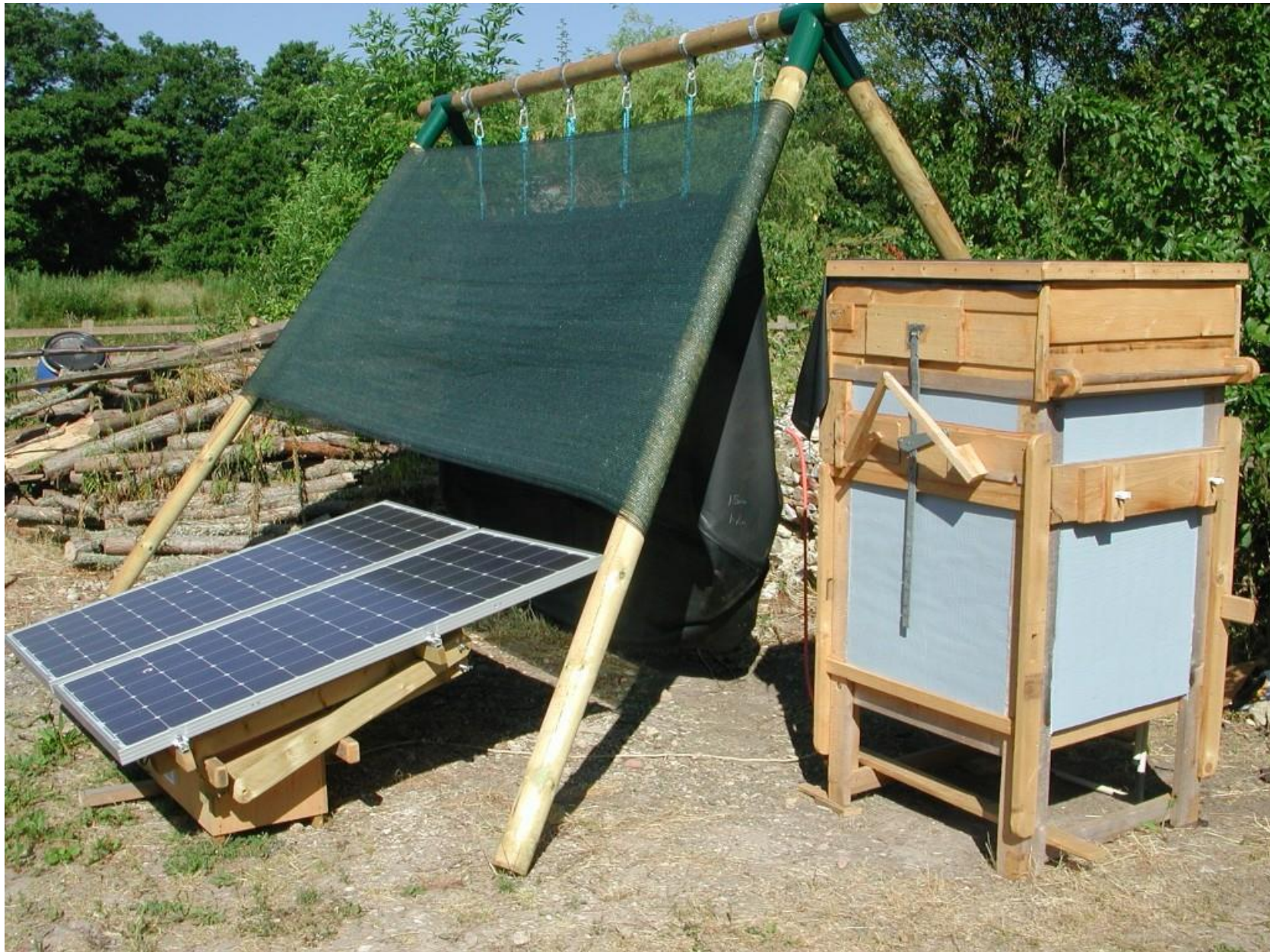
The AD system installed at Trill. The digester on the right is of 220 litres capacity, the bladder (behind the sun screen) a nominal 3 cu M, and the pv station 380 Wp.
