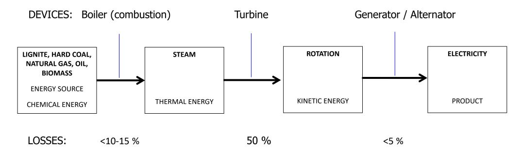
**EFFICIENCY** is the sum of effectivity of all energy transformation processes, in the picture above it is calculated as  $100 \times 0.85 \times 0.5 \times 0.95 = 40.375\%$
