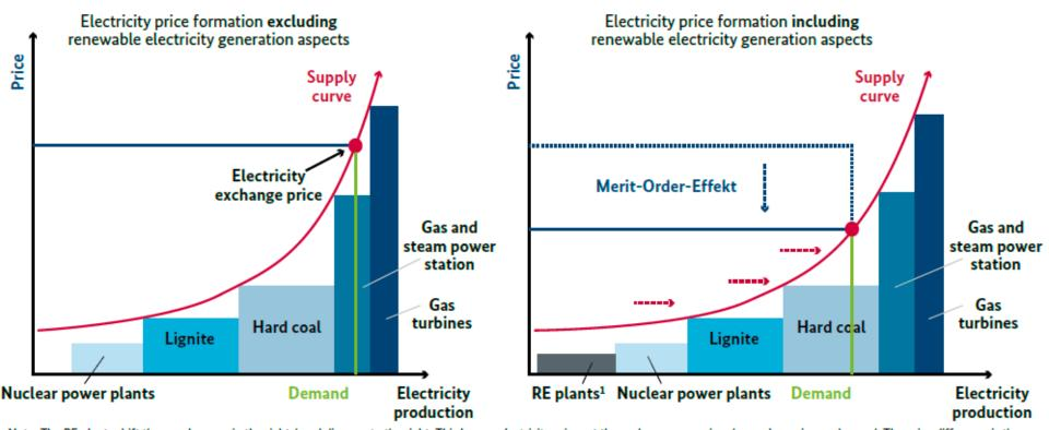
Note: The RE plants shift the supply curve in the right-hand diagram to the right. This lowers electricity prices at the exchange, assuming demand remains unchanged. The price difference is the merit-order effect.
