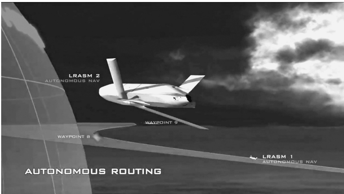
While en route to their human-designated targets, the LRASMs employ autonomous routing around pop-up threats (shown as a bubble).
