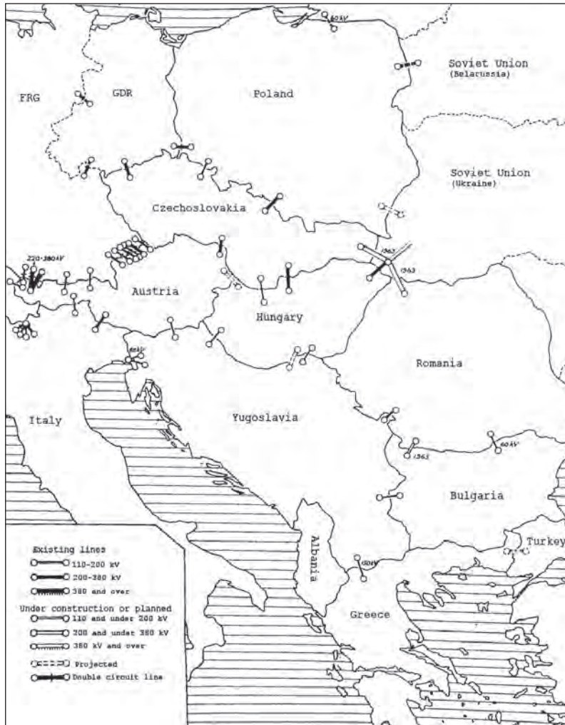
Figure 5.6 – Existing and planned cross-border interconnections in Central Europe in 1963 Source: UNECE, Outline of a Study on the Possibilities of Increasing Interconnexion Between Electric Power Transmission Networks in Europe, UN doc. ser., ME/31/64/C.2(a) (Geneva: UNECE, 1964).
