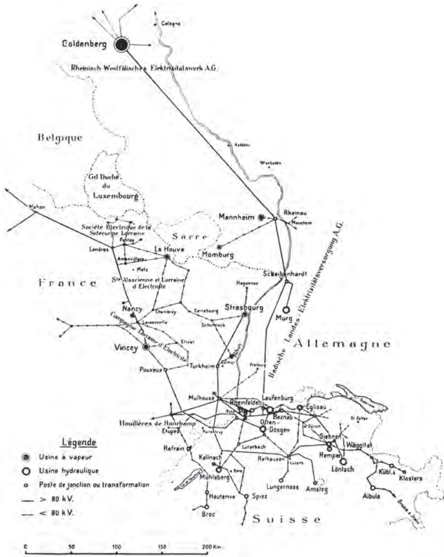
Figure 2.1 – Swiss, French, and German interconnections around in 1926 Source: H. Niesz, 'L'Échange, 1026. Used by permission of the World Energy Council, London, www.worldenergycouncil.org .
