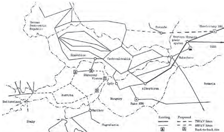
Figure 5.8 – Cross-border HVDC connections and 400-750 kV lines in Central and Eastern Europe, existing and proposed in 1985
