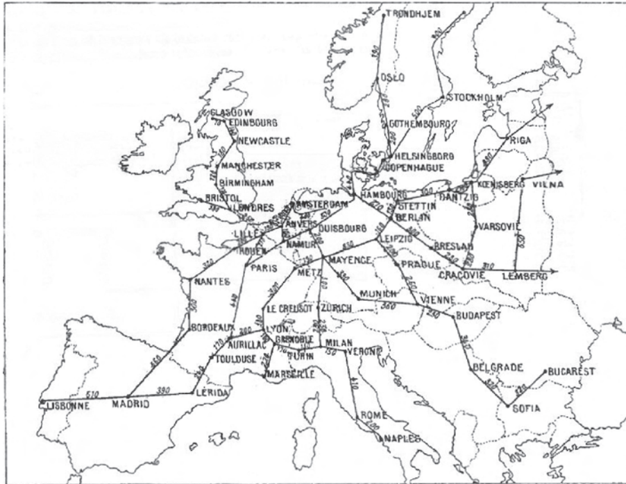
Figure 3.3 – George Viel's 400 kV network for Europe Source: Viel, "Étude," 743, figure 14.
