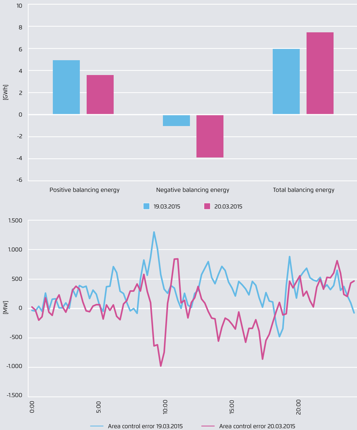
Comparison of activated balancing energy (top figure) and the remaining area control error (bottom figure) in the German power grid on 19 and 20 March 2015
