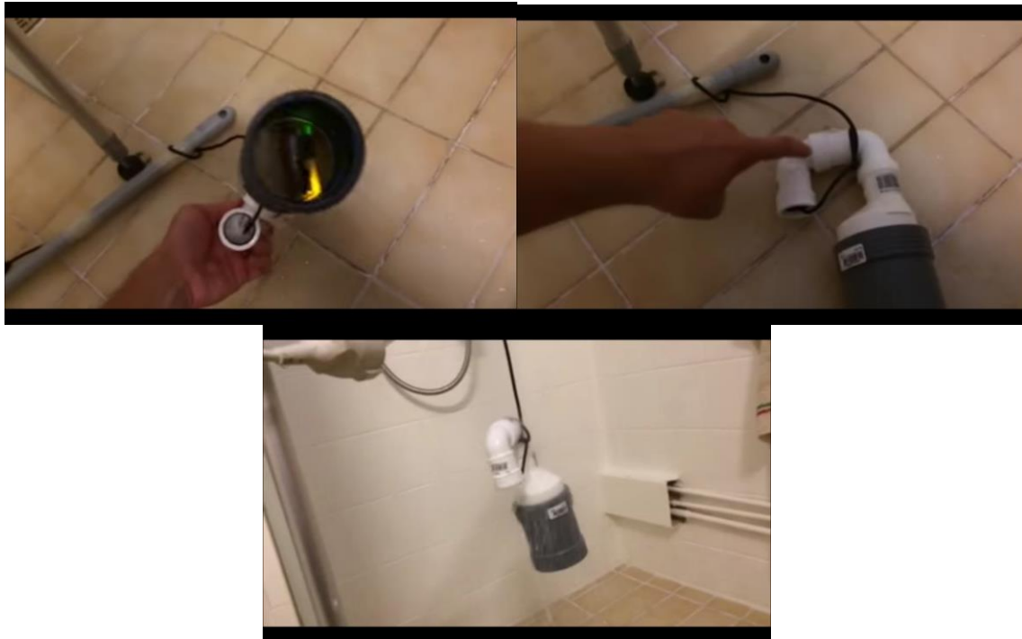
Figure 2 Screenshots showing the prototype of a drain-pipe housing for the Smart Citizen Kit
