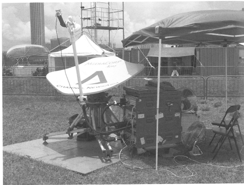
Figure 24.4 The mobile satellite dish is also sometimes called a Fly-Away system which can be moved between locations at short notice. They have been used everywhere from Everest to the heat of a desert. (Courtesy: Channel NewsAsia Singapore)
