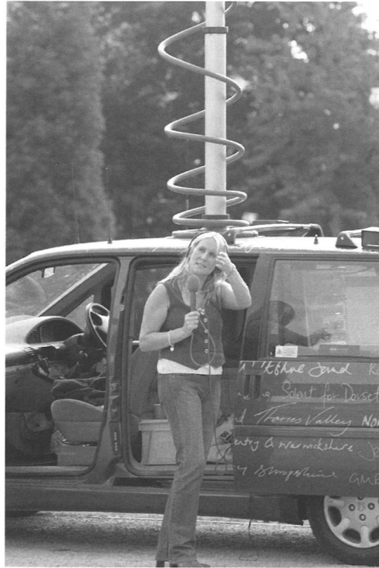
Figure 18.2 The radio car with its tall pump-up aerial acts like a mobile studio for sending on the spot reports back to the station. The idea is to keep the operation as simple as possible so that a story can be covered without the need of an engineer. (Courtesy: Katherine Adams/BBC)
