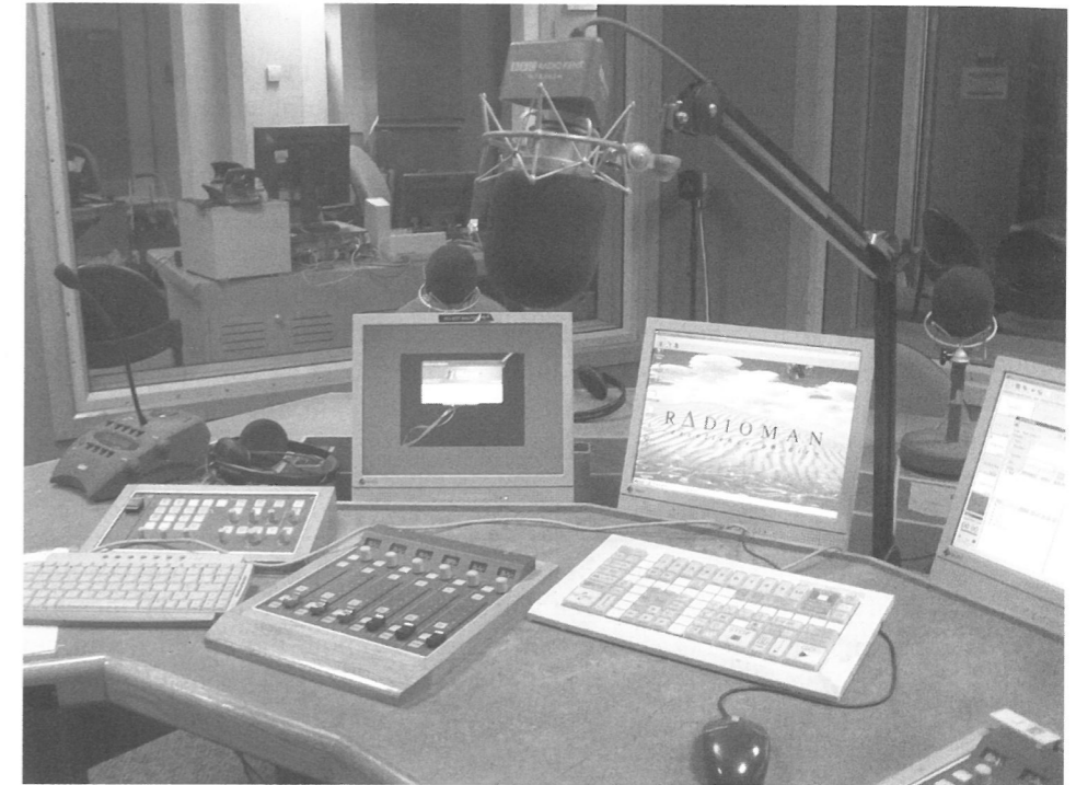
Figure 18.1 A self-opped presentation studio, with line-of-sight to a producer through the glass on the left, and a mirror-image studio through the other pane. (Courtesy: BBC/Peter Stewart)
