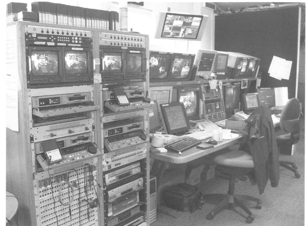
Figure 13.2 'The Hub' where pictures come in from remote studios, the satellite truck or Television Centre in London. (Courtesy: BBC/Peter Stewart)
