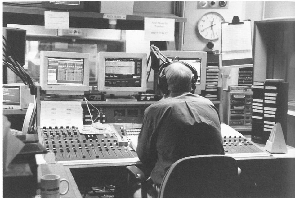
Figure 21.1 Catering for every form of audio, old, new and emerging – computers, phone, CD, cart, record and tape decks, all input through the mixing desk. (Andrew Boyd)
