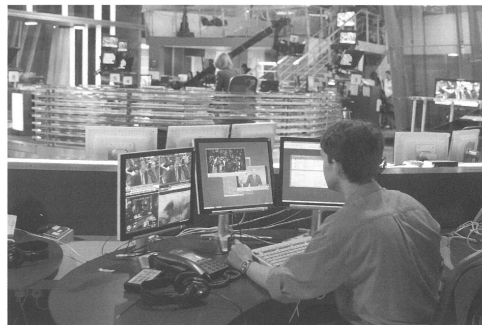
Figure 22.2 Television presentation, production, journalism and technology in partnership. The main component now is a large central server into which all sound and pictures, packaged reports, agency feeds and archive are ingested for instant access on desktop stations. (Courtesy: Sky News)
