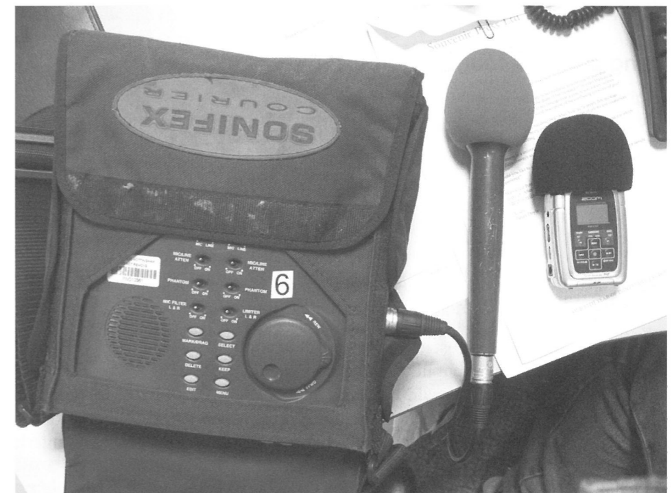
Figure 19.2 The new and the even newer. The flash-card technology of the Courier, and the Zoom H2 portable recorders, which is literally pocket-sized. Indeed the mike of one is larger than the whole Zoom device. (Peter Stewart)
