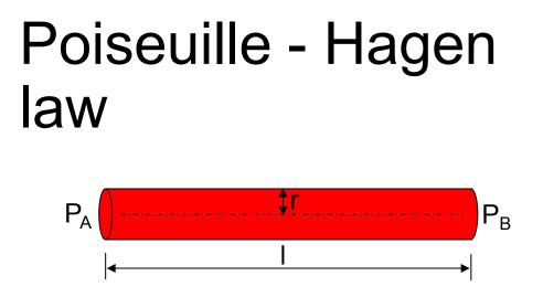
*Volume flow (Q)* in rigid tube equals directly to pressure gradient between beginning and end of the tube ( $\Delta P = P_A - P_B$ ), the fourth power of its radius (*r*) and indirectly to its length (*I*) and viscosity of the fluid ( $\eta$ )
