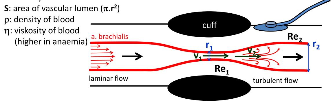
closely behind narrowing of the artery:  $S_1 < S_2$  a  $v_1 \approx v_2 \rightarrow Re_1 < Re_2 \rightarrow$  turbulent flow
