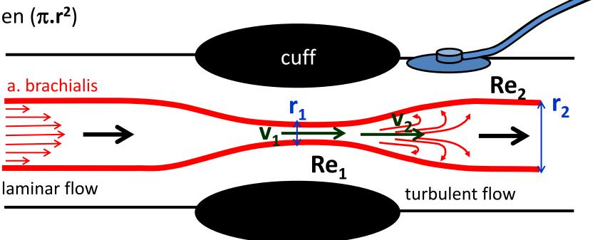
closely behind narrowing of the artery:  $S_1 < S_2$  a  $v_1 \approx v_2 \rightarrow Re_1 < Re_2 \rightarrow$  turbulent flow
