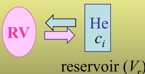
*Principle of method:* 1 Maximal expiration, 2 Repeated inspiration from and expiration into a reservoir (known volume  $V_r$ ) with inert gas  $He$  (known concentration  $c_i$ )
