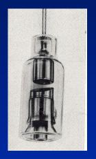
Catode (heated) - Electrons – go against Anode – brake - x ray originates
