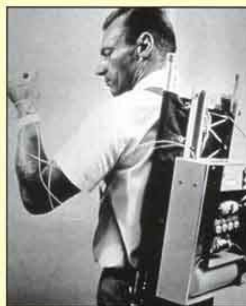
LEFT: The earliest protoType of an insulin pump which also delivered glucagon. Whitehall Laboratory, Indiana, 1963. RIGHT: 14-year-old Canberra pump-wearer, 2002. The device weighs 100g.
