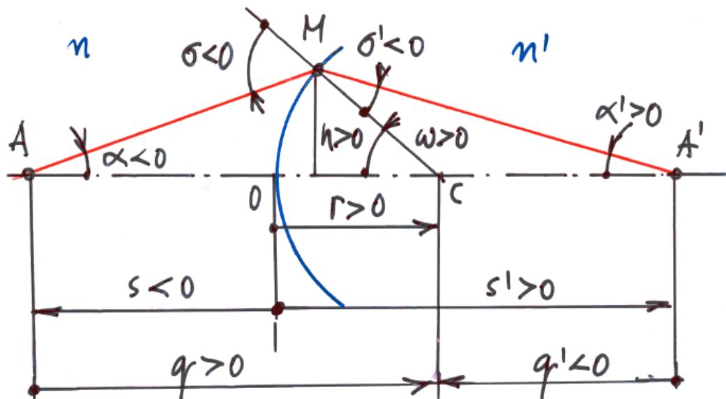
$$\begin{aligned} \sin \sigma &= \frac{q}{r} \sin \alpha, & \sin \sigma' &= \frac{n}{n'} \sin \sigma, \\ q &= r - s, & q' &= r \frac{\sin \alpha'}{\sin \sigma'}, \\ \alpha' &= \alpha + \sigma' - \sigma, & s' &= r - q'. \end{aligned}$$
