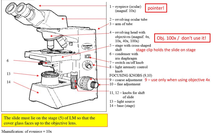
of objectives = 4x, 10x, 40x, immersion objective = 100x
