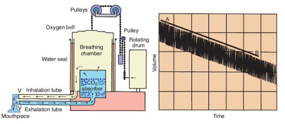
**FIGURE 27–8** Diagram of a modified Benedict apparatus, a recording spirometer used for measuring human O<sub>2</sub> consumption, and the record obtained with it. The slope of the line AB is proportionate to the O<sub>2</sub> consumption. V: one-way check valve.
