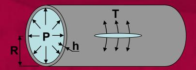
Considering thickness of vessel wall (h [m]): T=P•R/h [N/m²]
