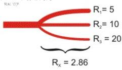
$$R_{x} = \frac{1}{\frac{1}{R_{1}} + \frac{1}{R_{2}} + \frac{1}{R_{3}}}$$
