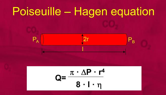
The flow of liquid in the cylindrical tube (Q) is directly proportional to the pressure difference between two ends of the tube  $(\Delta P = P_A - P_B)$ , to the fourth power of the tube radius (r) and inversely proportional to tube length (*I*) and to the viscosity of liquid ( $\eta$ )
