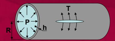
Considering thickness of vessel wall (h [m]): T=P•R/h [N/m<sup>2</sup>]
