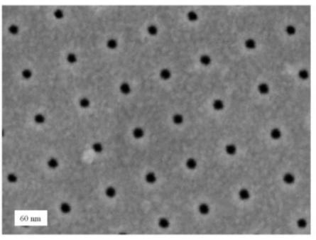
Solidstate nanopores drilled by a focused-ionbeam in a 10 nm thick silicon nitride membrane. The scale bar is 60 nm. Ref: H.D. Tong, H.V. Jansen, V.J. Gadgil, C.G. Bostan, J.W. Berenschot, C.J.M. van Rijn, and M. Elwenspoek, Nano Lett. 4, 283, (2004).
