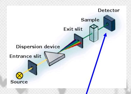
Light of one selected wavelength or whole transmitted spectrum can be measured
