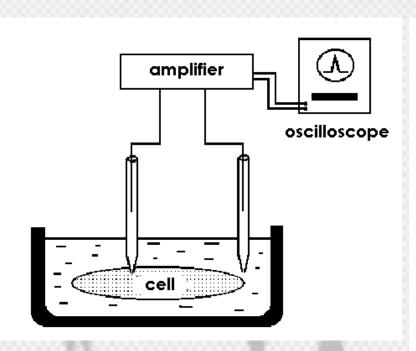
A blunt glass microelectrode clings to the surface of the cell or an isolated part of the biological or artificial membrane. The opening at the end of the microelectrode is completely sealed by the membrane "patch" and the measured electric voltages or currents thus relate to only a small part of the membrane, in which a small number of ion channels are found.
