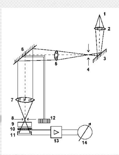
The **light source** (1) is a tungsten lamp. Its polychromatic light passes through a condensor (2) and reflects from a mirror (3) to the input slit (4) of the monochromator (parts 4 to 8, plus 12). The light is collimated (5) onto a reflection optical grating (6) which forms a colour spectrum. An almost monochromatic light is projected by an objective (7) onto the exit slit (8) of the monochromator.
