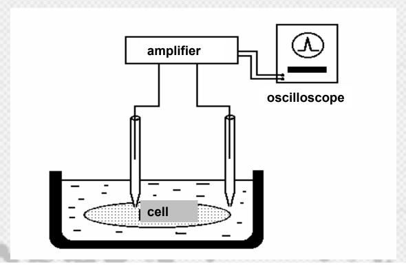
When using glass microelectrodes, it is possible to measure also other electrochemical parameters of the cells and membranes, e.g., concentrations of some ions. They can be prepared as ion selective electrodes for Na<sup>+</sup>, K<sup>+</sup>, Ca<sup>2+</sup>, H<sup>+</sup> etc.
