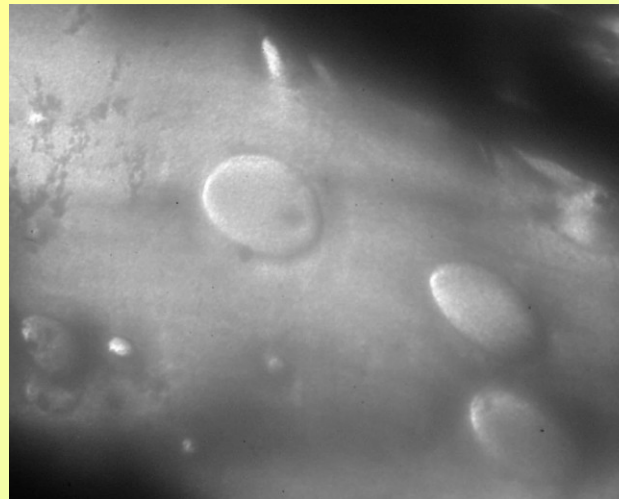
LV-TEM micrograph, crystals of polypropylene, frame width 6,3 \mu\text{m} , accelerating voltage 5 kV.
