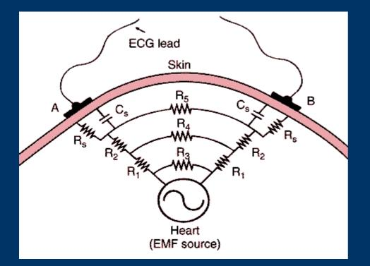
FIGURE 28–30 Why the ECG is so small. Multiple resistances and capacitances in the body decrease the potential and distort the waveform before the EMF reaches the surface.
