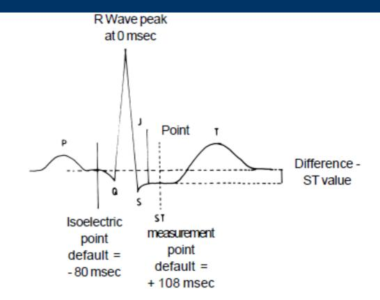
Fig - 4 : Adjustable reference points for automated ST segment analysis
