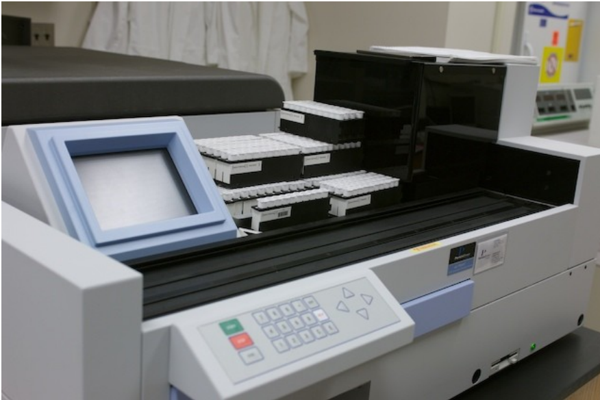
a 10-channel, 1000-sample PerkinElmer Wizard 1470 gamma counter
