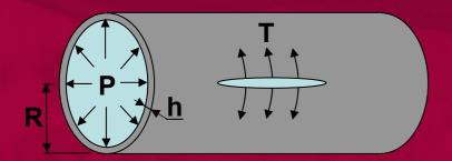
Considering thickness of vessel wall (h [m]): T=P·R/h [N/m²]
