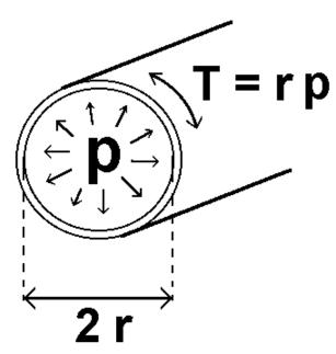
Laplace law – mechanical stress of blood vessel walls is directly proportional to the pressure and **vessel** radius
