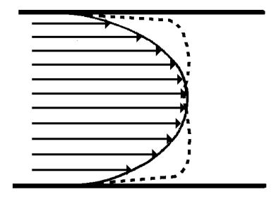
The differences between theoretical and real flow rate profiles are given mainly by the fact that blood is a non-Newtonian liquid and is influenced by the distensibility and compliance of the vessel wall..
