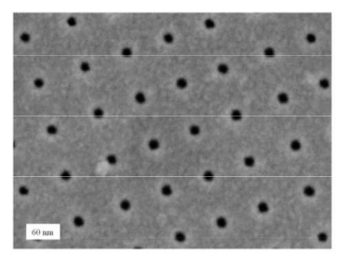
Nanopores drilled by a focused-ion-beam in a 10 nm thick silicon nitride membrane. The scale bar is 60 nm.
