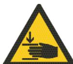
Warning, crushing hazard: hand (Standard ISO 7010).
