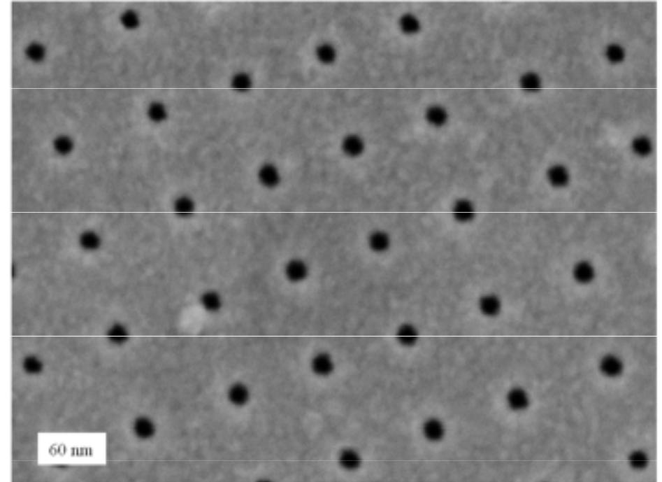
Nanopores drilled by a focused-ion-beam in a 10 nm thick silicon nitride membrane. The scale bar is 60 nm.
