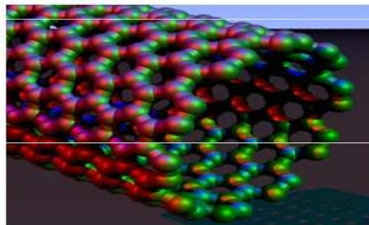
Depending on the structure of carbon nanotubes, the nanotube behaves as a metal or as a semiconductor (or even a superconductor!). See so called "Armchair Quantum Wire," elsewhere.
