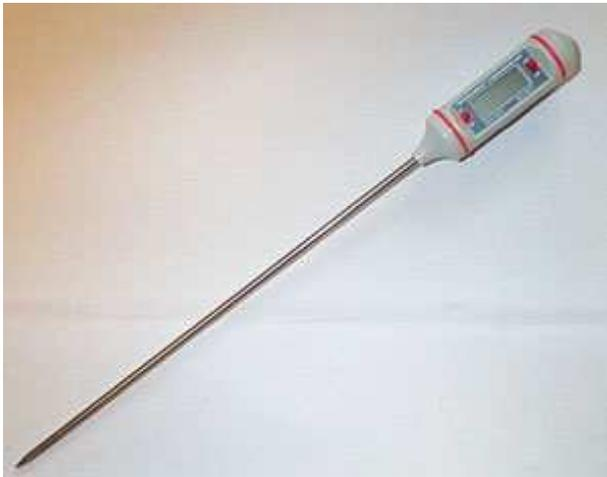
Digital thermocouple sensor
