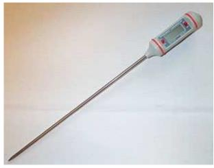
Digital thermocouple sensor
