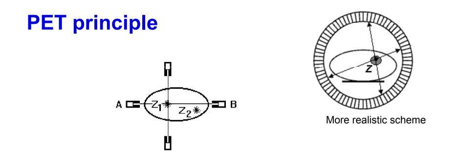
Explanation of the **high spatial resolution of PET**: The opposite detectors in a coincidence circuit. A source of radiation Z is detected only when lying on a line connecting the detectors. Detector A but not the detector B can be hit through a collimator from the source  $Z_2$ , because this source is outside the detection angle of B. In SPECT, the signal detected by A from  $Z_1$  would be partially overlapped by the signal coming from source  $Z_2$ .
