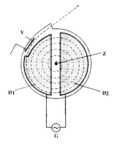
Z – source of the accelerated particles (protons),
