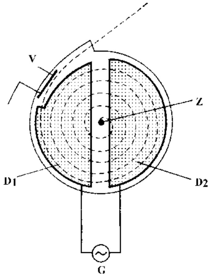
Z – source of the accelerated particles (protons),
