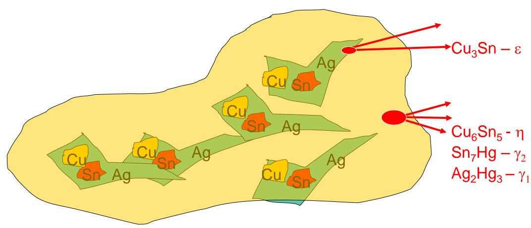
Gamma two disapears or it does not occur when content of copper is high
