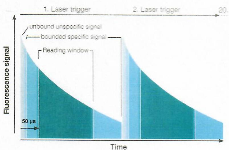
**Time resolved:** Short signals of unbound fluorophores are differentiated by a 50  $\mu$ s delay of reading window from the long signal of the bound immunocomplex. This long-lived signal is proportional to the concentration of the analyte of interest.
