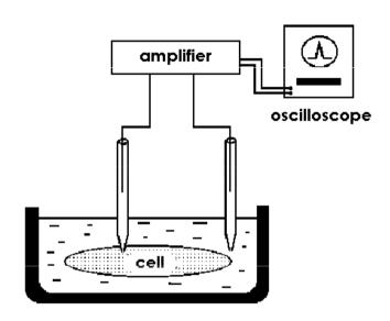
A blunt glass microelectrode clings to the surface of the cell or an isolated part of the biological or artificial membrane. The opening at the end of the microelectrode is completely sealed by the membrane "patch" and the measured electric voltages or currents thus relate to only a small part of the membrane, in which a small number of ion channels are found.
