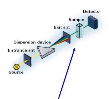
Light of one selected wavelength or also whole transmitted spectrum can be measured
