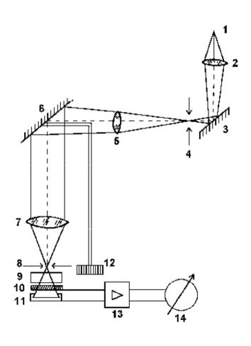
The **light source** (1) is a tungsten lamp. Its polychromatic light passes through a condenser (2) and reflects from a mirror (3) to the input slit (4) of the **monochromator** (parts 4 to 8, plus 12). The light is collimated (5) onto a **reflection optical grating** (6) which forms a colour spectrum. An almost monochromatic light is projected by an objective (7) onto the **exit slit** (8) of the monochromator.
