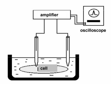
When using glass microelectrodes, it is possible to measure also other electrochemical parameters of the cells and membranes, e.g., concentrations of some ions. They can be prepared as ion selective electrodes for Na<sup>+</sup>, K<sup>+</sup>, Ca<sup>2+</sup>, H<sup>+</sup> etc.
