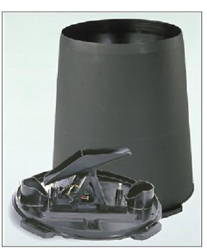
A rain gauge measures the depth of water (in millimeters or inches) precipitated over a level surface. It should be sited away from barriers that could create wind effects to prevent wind from blowing rain into or around the gauge. Snow can present some problems especially if the gauge is not well screened and wind blows the snow around. In addition, large depths of snow may exceed the opening of the gauge before it can melt and therefore be measured.
