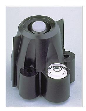
Solar radiation, measured using a solarimeter, is observed as a total of all wavelengths although in some specialized automatic weather stations, specific wavelengths may be monitored.
