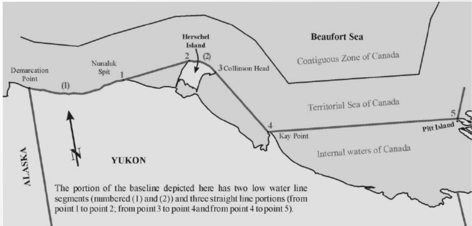
The portion of the baseline depicted here has two low water line segments (numbered (1) and (2)) and three straight line portions (from point 1 to point 2; from point 3 to point 4 and from point 4 to point 5).
