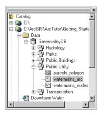
Watermains\_arc is a feature class—a collection of features represented with the same geometry (shape). In this case, the features are polyline shapes that represent the pipes in the water distribution system.
