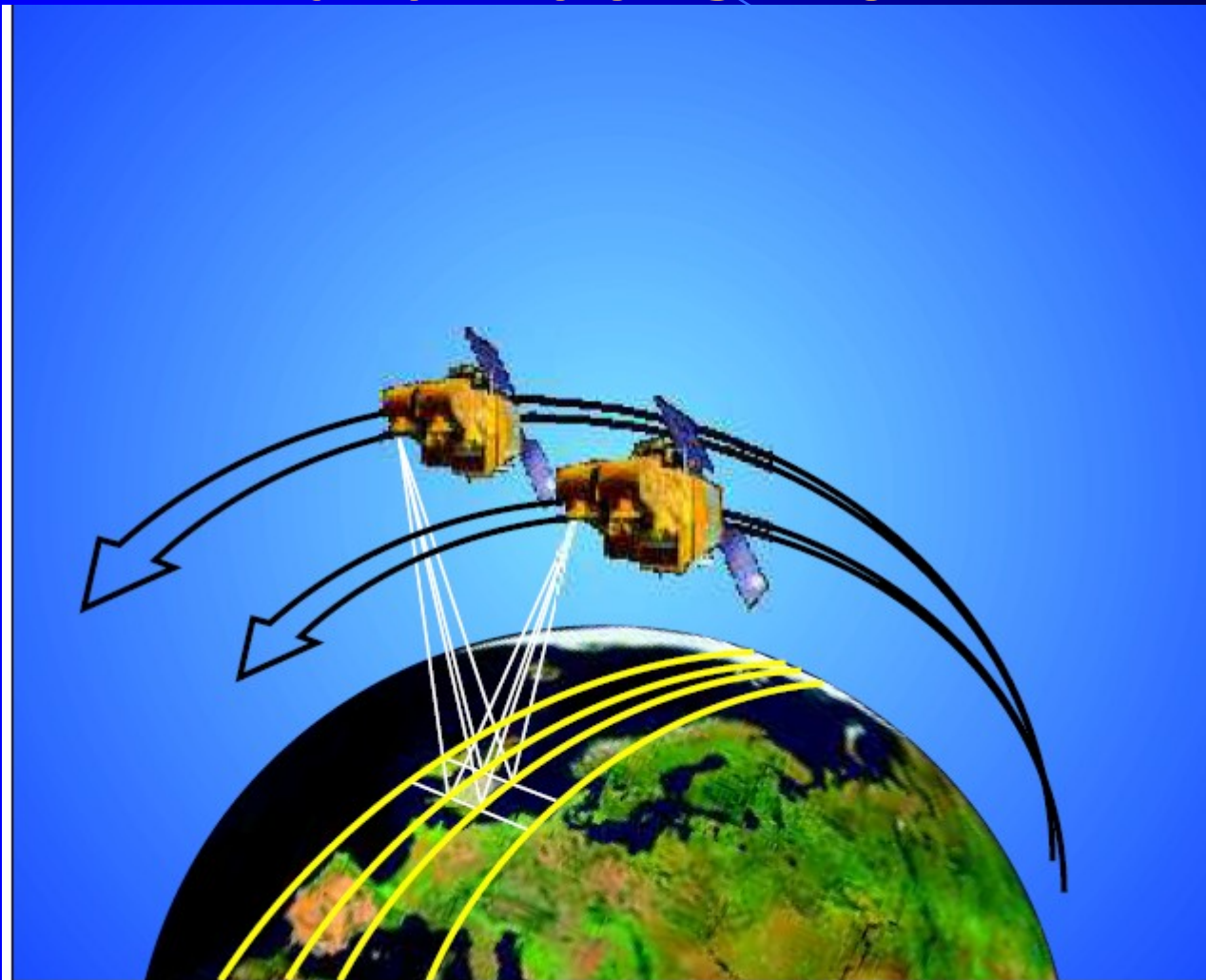
4a. Scanning of SPOT stereo images at neighbour overflight.
