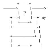
If ny and nu "consume" all inputs and outputs of K then the result is a lower fractional transformation. If ny and nu "consume" all inputs and outputs of P then the result is an upper fractional transformation.
