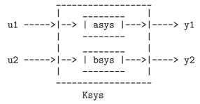
The function also rearranges the internal state-space realization of sys so that the continuous states come first and the discrete states come last. If there are duplicate names, the second name has a unique suffix appended on to the end of the name.
