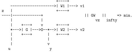
The closed loop system GW from [z; u]' to [v1; v2; y]' can be obtained by (all SISO systems):
