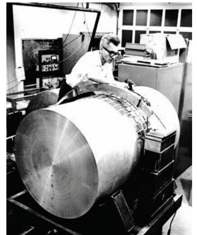
Figure 7.20 Joseph Weber and his resonant bar detector.
