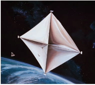
Figure 2.8 Solar sails have been proposed as a form of spacecraft propulsion. They are propelled by the momentum of photons.
